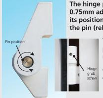
The hinge pin and polymer hinge bearing are both acentric and allow for +/-0.75mm adjustment each to the hinge position. The dot on the top of the pin shows its position and this can be adjusted with an allen key inserted into the bottom of the pin (release the grub screw in the hinge to allow adjustment).
